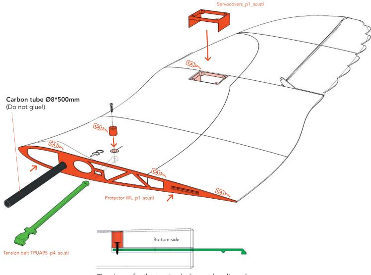
The sleeve for the tension belt must be aligned as shown here so that the belt can be secured with a screw.
