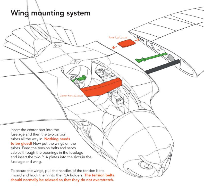
Do not worry, if the tension belts are not hooked in, the canopy cannot be closed. So you don't forget to secure the wings before the flight.
