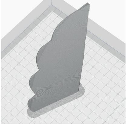
The following parts must be sliced with the PROFILE P5\_GYROID. Please note the additional settings for the individual parts! It is essential to print these parts with LW-PLA!
