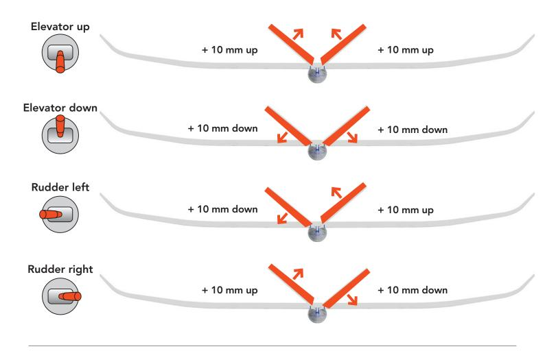
At full throttle the nose pulls up a bit, to avoid this you can mix some elevator down to the trottle (about 10%). But do not test this at the first start but at high altitude!
