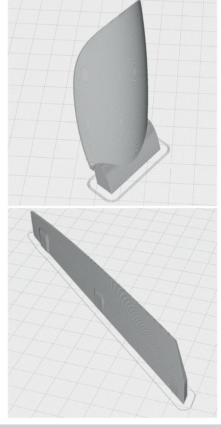
The following parts must be sliced with the PROFILE P5\_Gyroid. Please note the additional settings for the individual parts! It is essential to print these parts with LW-PLA!
