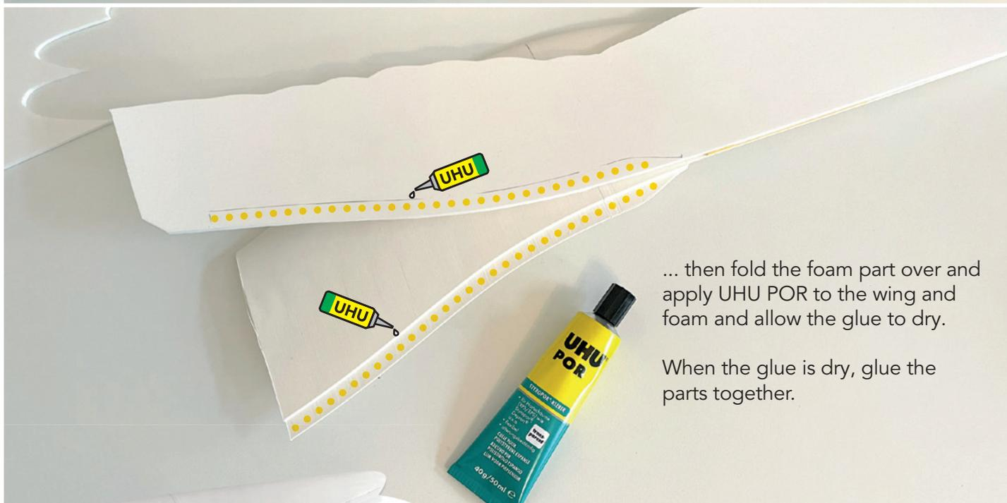
... then fold the foam part over and apply UHU POR to the wing and foam and allow the glue to dry.
