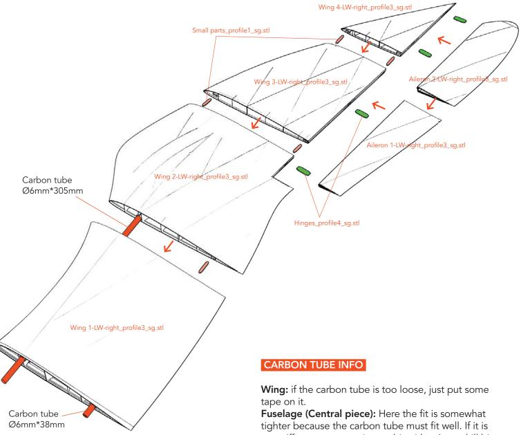
**Fuselage (Central piece):** Here the fit is somewhat tighter because the carbon tube must fit well. If it is too stiff, you can open it up a bit with a 6mm drill bit. You can also use a piece of carbon tube as a drill. Due to the frictional heat, the PLA adapts.
