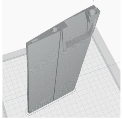
The following parts must be sliced with the PROFILE P5\_GYROID. Please note the additional settings for the individual parts! It is essential to print these parts with LW-PLA!
