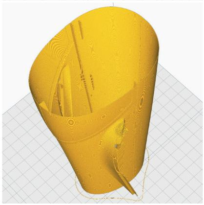
The following parts must be sliced with the Funktion **Spiralize Outer Contour** (Cura) or **Spiral Vase** (Prusa Slicer). For these parts, only the outer wall (1 line/perimeter) is printed without Z-seam, no top and bottom layers. **It is essential to print these parts with LW-PLA!**
