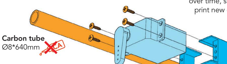
The servo is attached in the same way as the servos for the elevator and rudder.
