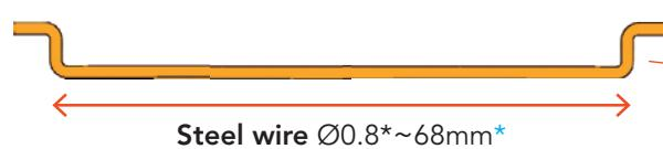
\*The exact length depends on the exact position of the servo lever you are using.
