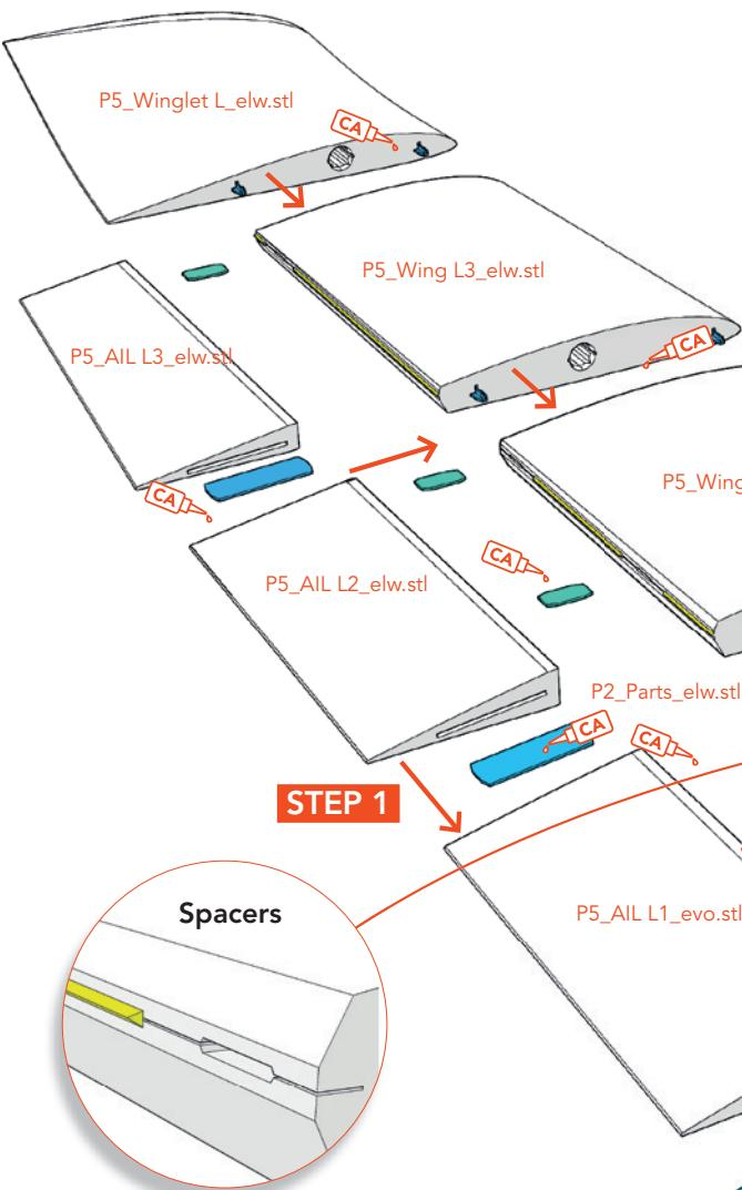
**Installation the TPU Hinges:** First insert the hinge into the **aileron** and add a drop of liquid CA adhesive into the gap. Wait for the glue to drain completely, then spray the activator on it. Then put the aileron in the wing **until it touches the spacers** and put a drop of CA glue on the hinge. Wait again for the glue to run in, and then spray the activator on it.
